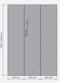
Fastening points for use on a stud frame with 300 mm stud spacing. Construction board thickness at least 10 mm.
