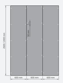
Fastening points for use on a stud frame with 600 mm stud spacing. Construction board thickness at least 20 mm.
