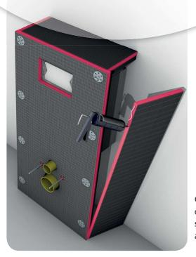
Clad the top and side parts of the WC wall frame using the other 2 boards, cutting them to size. These boards can be secured to the wall, floor and front cladding using a suitable assembly adhesive (e.g. solvent-free PU-based adhesive).
