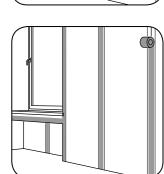
Glass-fibre tape or joint tape must be applied to all butt joints which should then be covered with two thin layers of filler.
