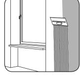
Apply a type flexible tile adhesive to the entire surface and fix to a level substrate (align if necessary).
